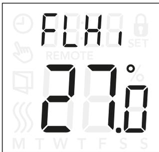
These settings allow you to set the minimum and maximum temperature that the thermostat can operate inbetween.
