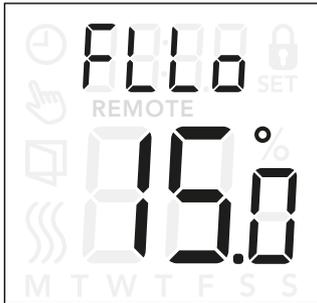
These settings allow you to set the minimum and maximum limits for the floor temperature, for example to protect sensitive floors..
