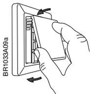
4. Align the top of the new front cover with the top of the thermostat.
