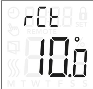
This setting allows you to set the temperature setpoint for the thermostat, when it is remote controlled.
