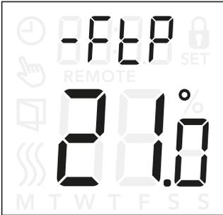
Depending on the type of sensor and sensor application setting, the temperature from the floor sensor (-FŁP) and the internal room sensor (-rŁP) can be monitored here.
