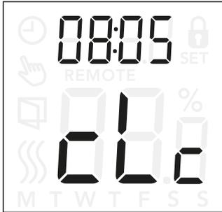
This option allows you to set the time. The time settings is used to control the event during scheduled operation.
