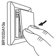
5. Press at the bottom of the new front cover to close.
