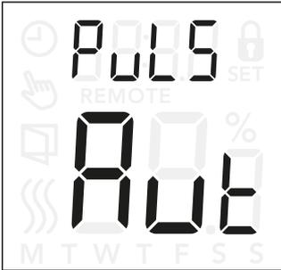
**Auto:** Similar to “PWM On”, but the PWM period is increased or decreased depending on the minimum and maximum temperature measured during a PWM period. This will increase the lifetime of the relay by reducing the number of relay switches, and still ensure the comfort of the user by keeping temperature fluctuations below an acceptable level.
