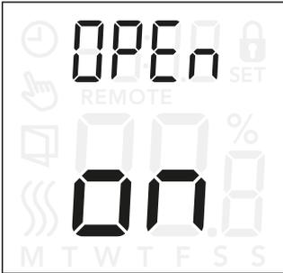
This setting allows you to enable the "Open window" function.
